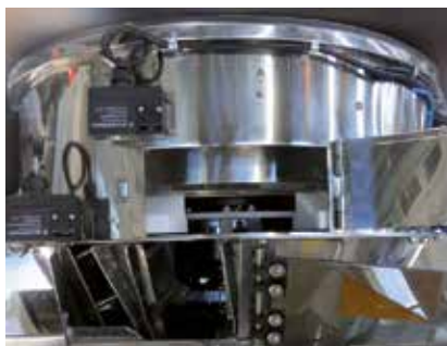
Access door to selectors and funnels to make the changeover
