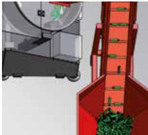
Bottles hopper elevator
