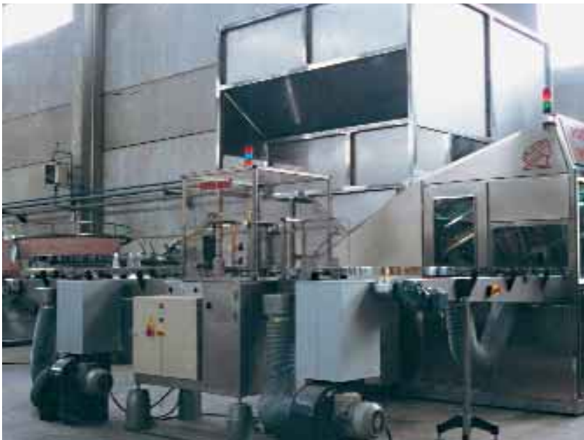
Silo Posisilo, Posimat unscrambler and Giramat orientor
